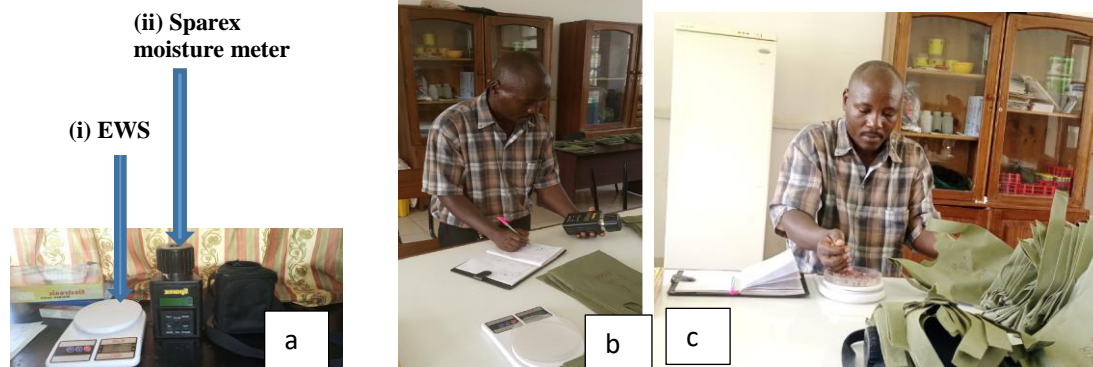
Plate 3.5: Electronic weighing scale and sparex moisture meter (a) Recording bean moisture content (b) Weighing bean seeds on electronic weighing scale (c).
